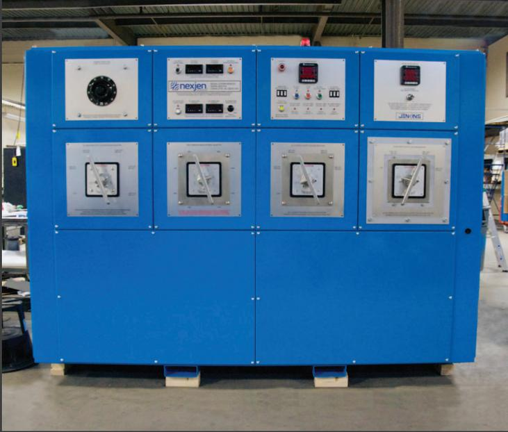
Nexjen Electric Motor Test Systems are built on the principle of safe, simple operation and dependable service. The same Jenkins test transformer design we have used for the past fifty years sits at the core of a power supply engineered to perform continuously at full ratings for 8 hours. With heavy duty components and very few moving parts, the Nexjen Electric Motor Test System is designed to operate for decades without maintenance.
